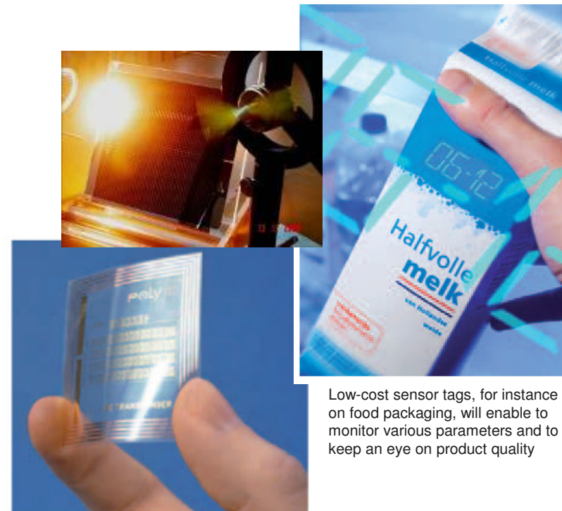
Model of a polymer flexible RFID-tag. Source: Polylc
